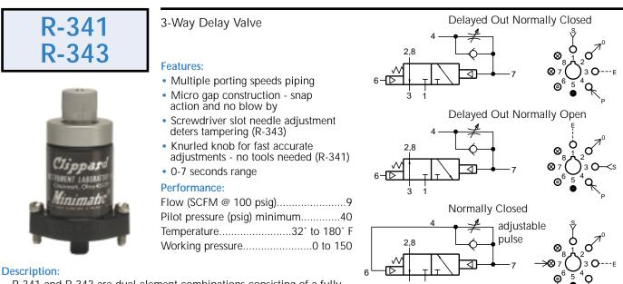
R-341 and R-343 are dual element combinations consisting of a fully ported spring return, 3-way valve and an adjustable flow control to provide a delay "out" function.
